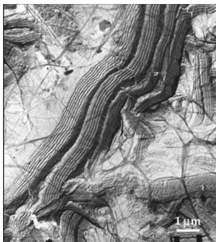
Fig. 6 Bands on the free surface of compacted PTFE dispersion particles sintered at 380 °C followed by slow cooling. (Similar to Fig. IV-65 in Ref. [4])
